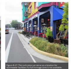
Figure B-27: The curb zone can serve as a location for stormwater facilities if a full frontage zone is not available.
